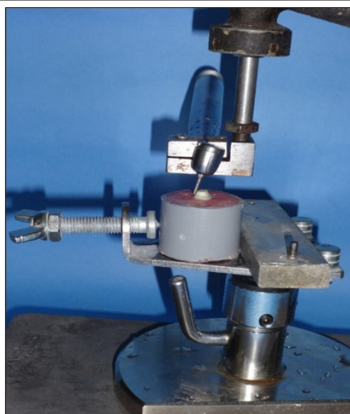
Figure 2. Tooth preparation with customized device
